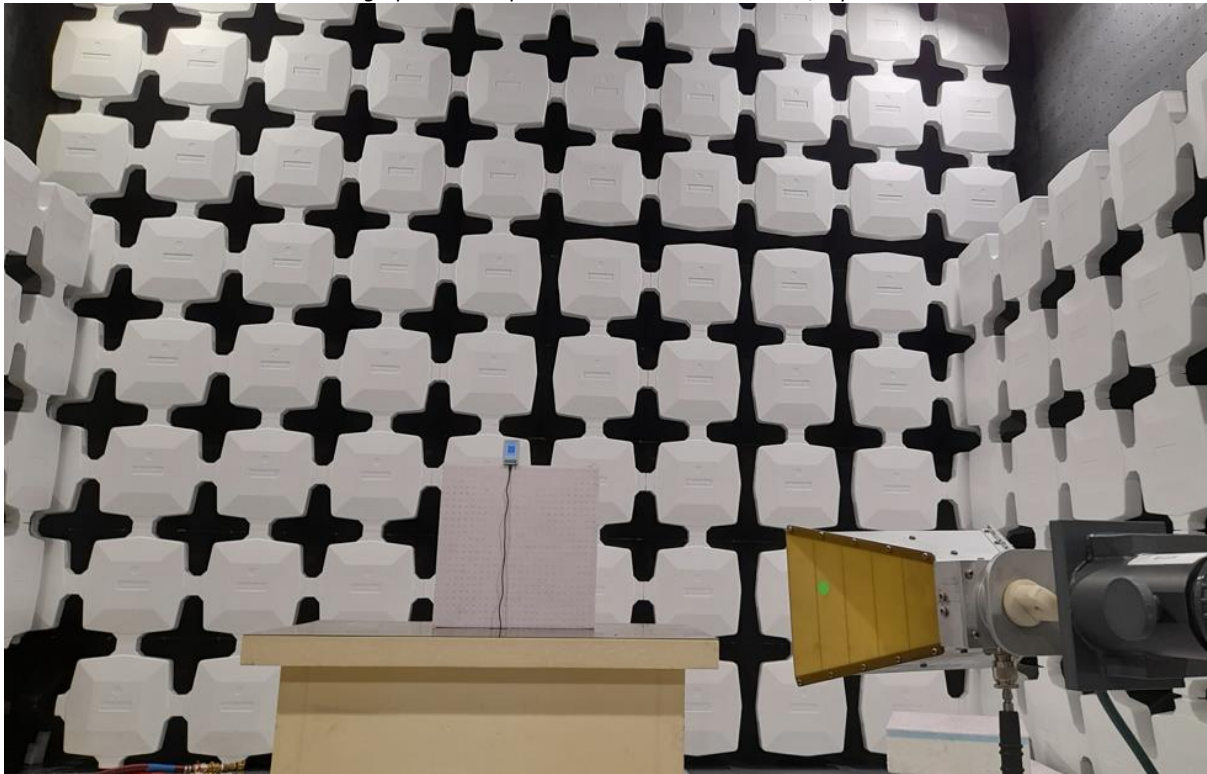
Photo 2 Photograph test setup radiated emissions 1-18 GHz, report section 3.1
